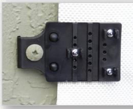
Nylon one-piece clips securely retain fabric with only 3 #14 x 3/4" sheet metal screws
